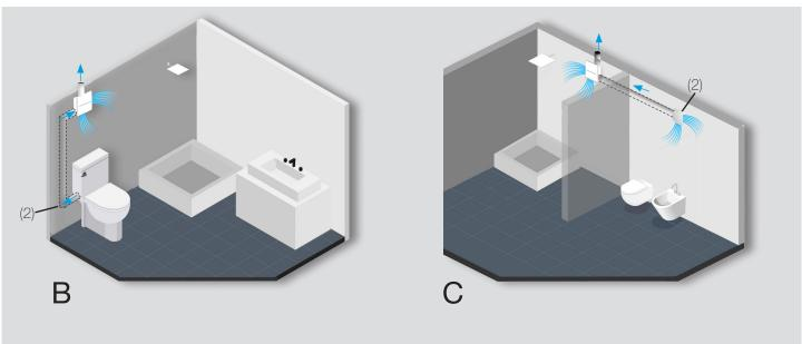
**B.** Example of additional air extraction (2) from the toilet bowl in combination with the standard front air intake.
